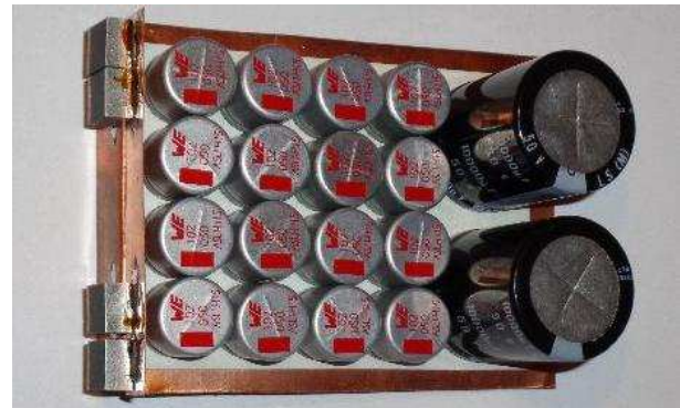
Fig. 8 Layout of the inductance-less battery of capacitors.
