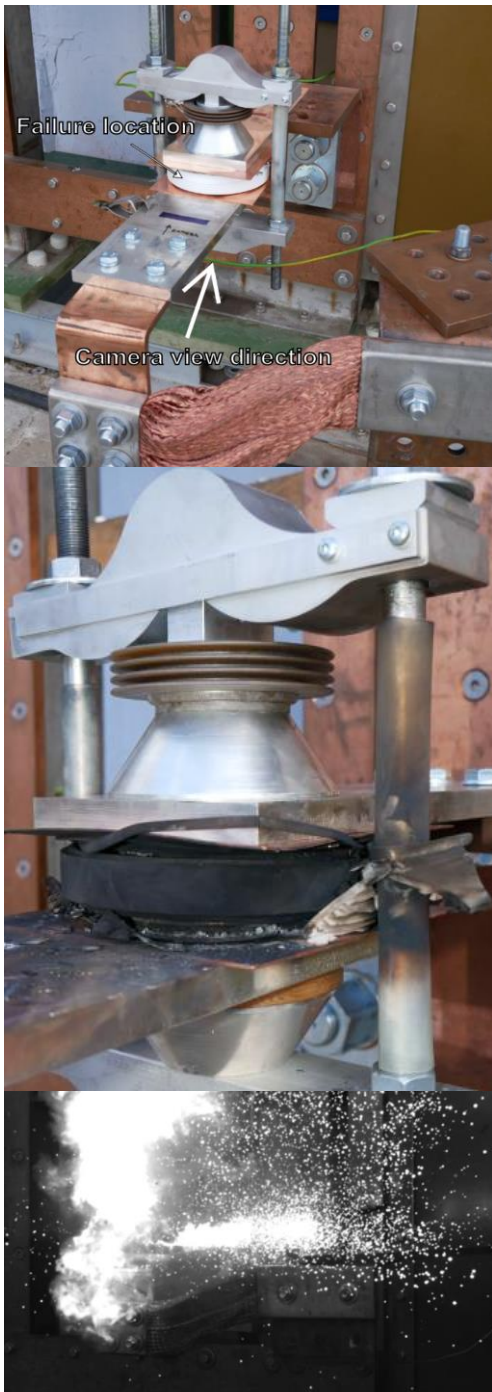
Fig. 10: Test setup in KEMA Labs in Prague (top), destroyed clamped housing where both key features were made from polymer (current approx. 85 kA) (middle), massive plasma escape captured on high-speed camera (bottom).
