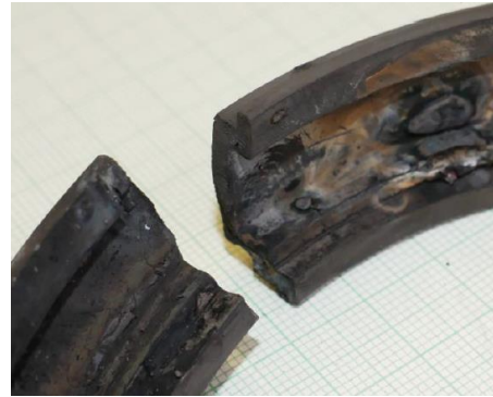
Fig. 8: Brittle fracture on polymer protection ring with too high reinforcement filling caused by massive pressure increase in the housing during reverse short-circuit failure.
