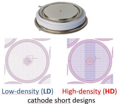
Fig. 1 Device under test: 5STP 08F6500 rated to V_{DRM} = 6.5 kV, I_{TAVmax} = 850 A. Two cathode designs: low-density (LD) and high-density (HD) cathode short pattern.
