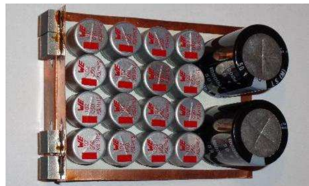
Fig. 8 Layout of the inductance-less battery of capacitors.
