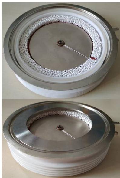
Fig. 14: Assembly with an additional ceramic foam ring (top) and the whole assembly with mounted protection disc but without a housing lid or cathode pole-piece (bottom).
