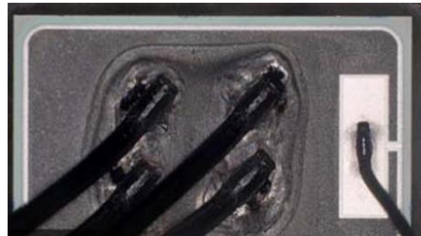
Fig. 4 Top view of decapsulated DUTs after surge current tests [3].
