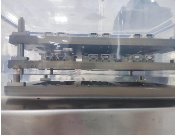
Figure 7: Setup for the soaking experiment with tested and new modules. An air sealed box is filled with water and stored in a climate chamber at 50 °C for 48 h.
