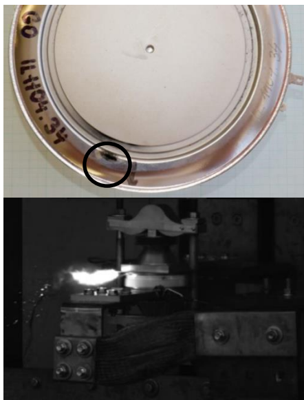
Fig. 13: Melted spot (circled) on top flange where the plasma escaped (top), photo from high-speed camera when I_{RSMC-MAX} is exceeded (bottom).
