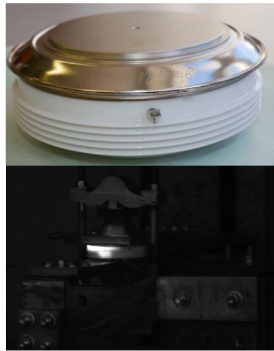
Fig. 11: Housing without hermeticity failure after 10 ms sinusoidal current pulse below or near I_{RSMC-MAX} (top), photo from high-speed camera during pulse below or near I_{RSMC-MAX} (bottom).
