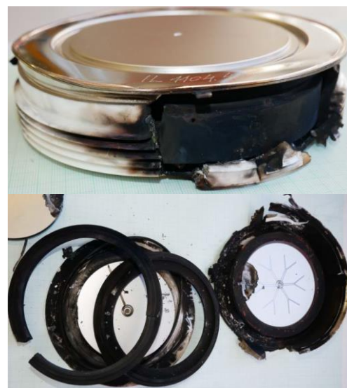
Fig. 9: Destroyed housing where both key features were made from polymer (current magnitude approx. 85 kA).
