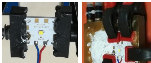
a) free convection air cooling b) forced water cooling
