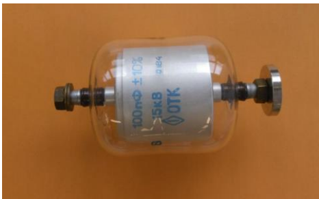
Figure 5: Vacuum capacitor used as an etalon.
